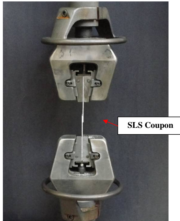
Figure 1 : SLS test set up and coupon configuration
